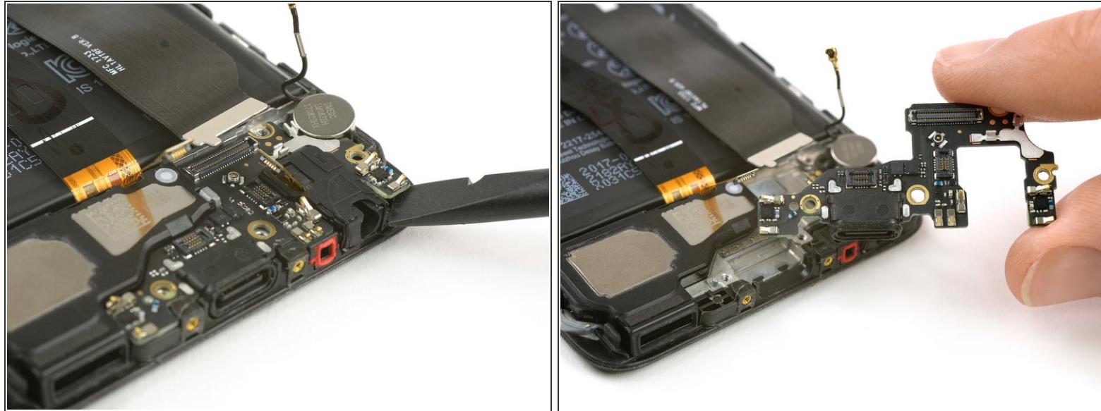
⚠ Do not damage any components sitting on the charging board while removing it.
